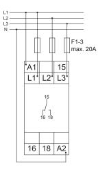
G2PW400V10 with power module 400V a.c.
